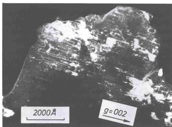
Fig. 2. Dislocations in shocked olivine from Apollo 11 (10085,26). Transmission electron micrograph. Dark field image produced by a reflection \vec{g} = 002 . Particle normal near [010]. Acceleration voltage 100 kV. (Siemens Elmiskope 101.)
